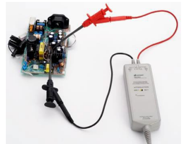
N2790A measuring a power supply signal
