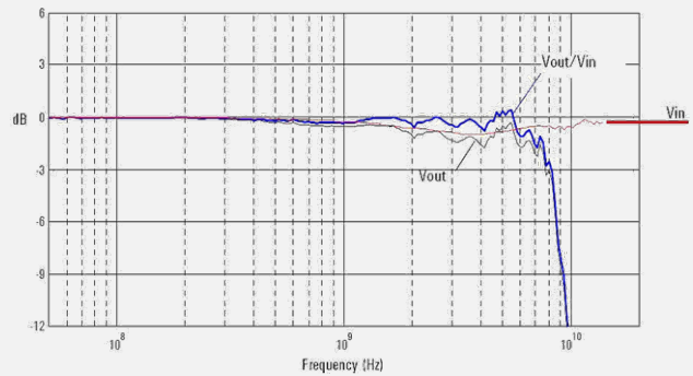
Swept frequency response with a 25- \Omega source
