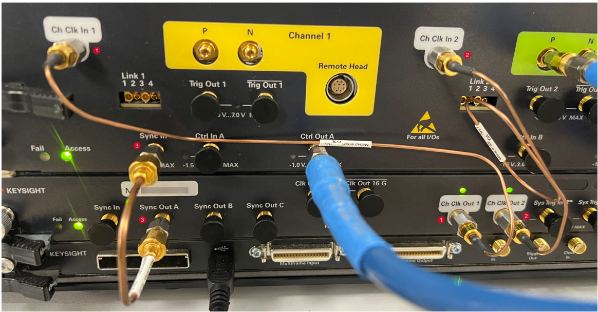
Figure 2 Using semi-rigid cables to connect M8009A and M8042A
