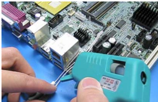
Figure 8 Probe Secured Using Low-Temperature Hot Glue
