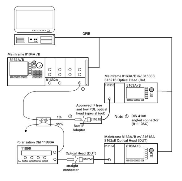
Figure 13 Measurement Setup for PDL Test
