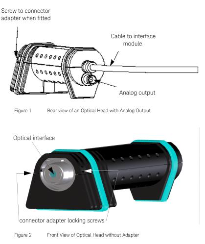
Figure 1 on page -17 and Figure 2 on page -17 show views of a typical optical head.
