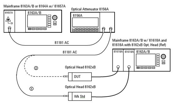
Figure 8 Accuracy Test Setup
