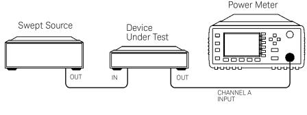
Figure 1-5 Limited checking application
