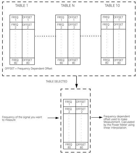
Figure 1-2 illustrates how frequency dependent offset tables operate.
