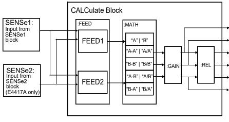
Figure 3-1 CALCulate block
