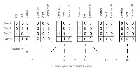
Figure 1-10 Typical status register bit changes
