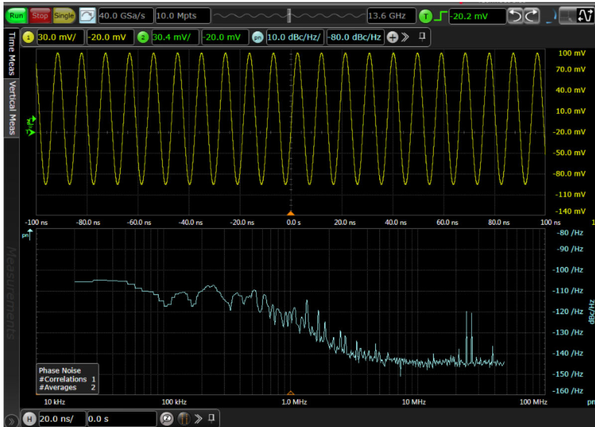
Figure 9. Using default settings, spurs in the spectrum are normalized into the plot.
