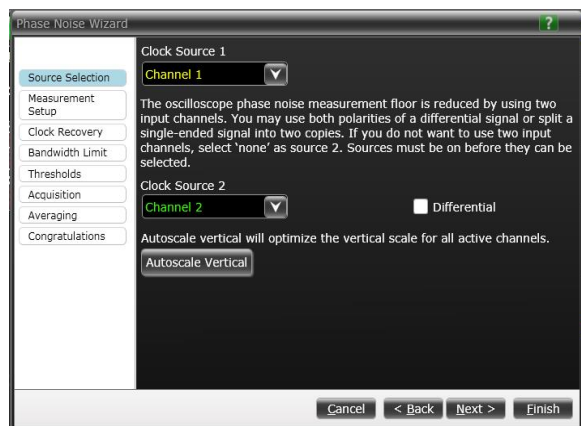
Figure 1. The measurement analysis wizard provides you instructions to help make the best decision of measurement options for the type of jitter
