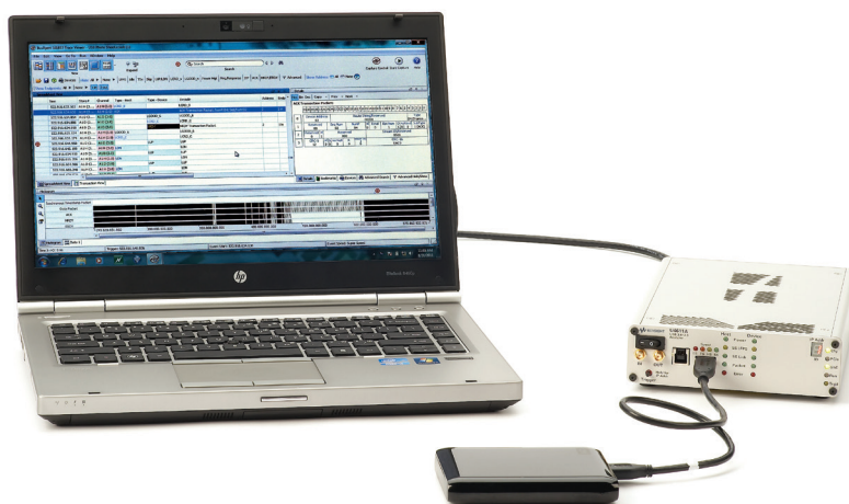
Figure 1. The U4611A/B Analyzer is connected in a pass-through mode and records traffic being exchanged between the host and the device under test.
