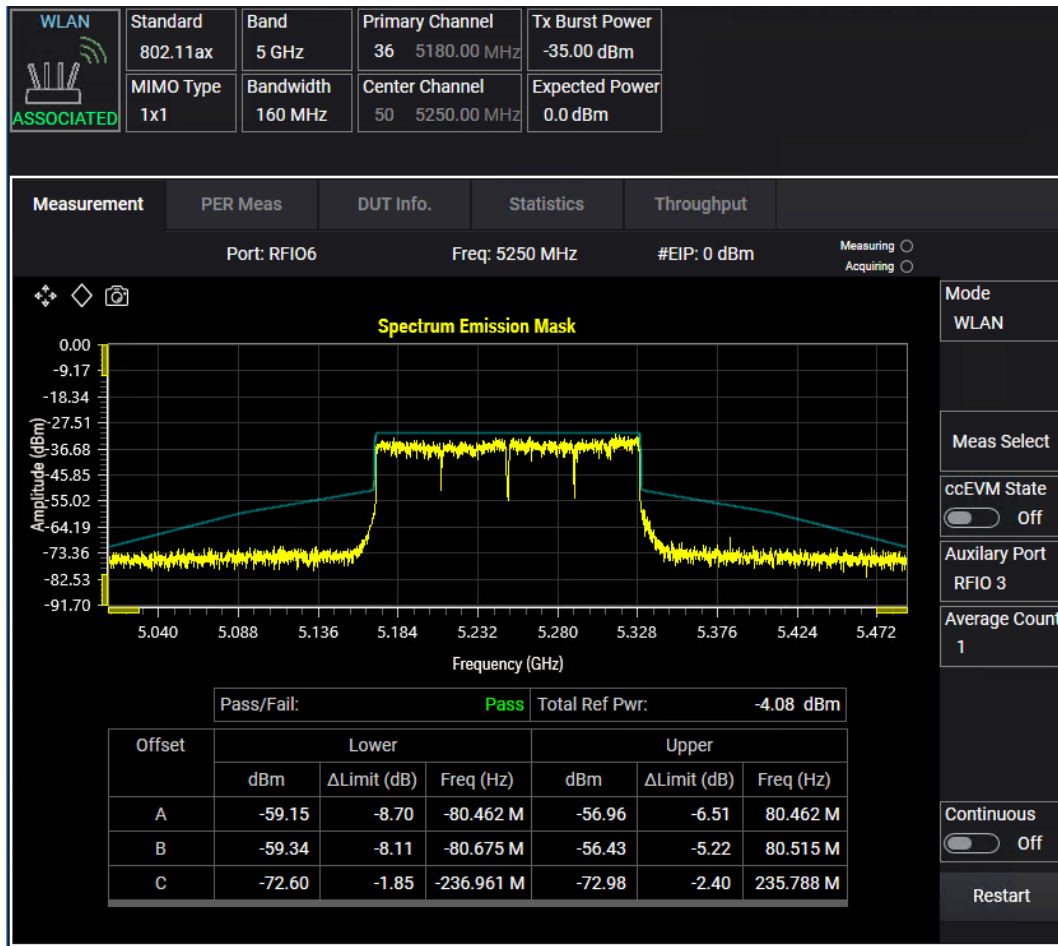
Figure 2. Example of spectrum emission mask measurement results for a Wi-Fi 6E client
