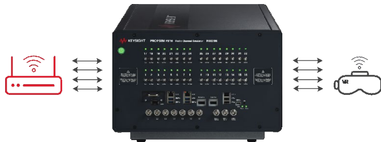
Figure 5. Lab setup example (FS16-16ch): Single-link operation using multiple resource units (RU) for single user is introduced in 802.11be. Setup to test 4x4 bi-directional 320MHz links
