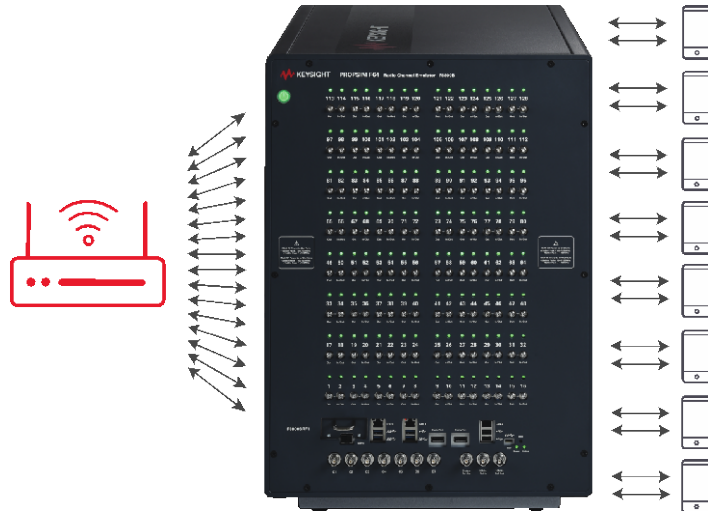
Figure 4. Lab setup example (F64-64ch): One 16x16 with bi-directional 160MHz links
