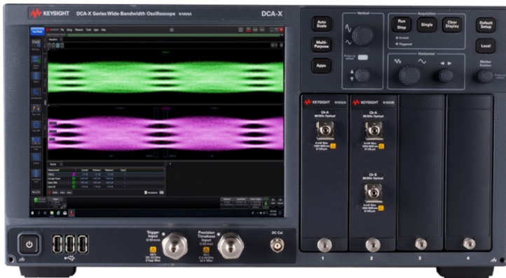
N1032A/B optical modules with N1000A DCA-X
