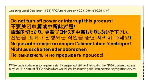
This Screen will appear and disappear for each LO board installed. It may appear as a Loop but it is dependent on the number of LO boards installed. Please be patient. The green progress bar will roll across the screen indicating software activity.
