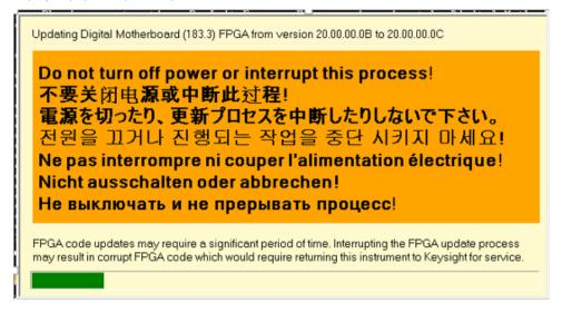
**NOTE:** The instrument is configured to have at least 3 LO boards installed. Updating the FPGA code on each board can take about 10 Minutes.
