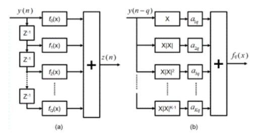
The structure of Volterra series is shown below. Volterra Series Structure
