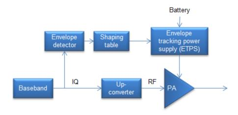
For envelope tracking PA, the envelope tracking power supply and the RF input signal should be aligned strictly in time. Even small time deviations will have substantial influence in the RF output signal, leading to the deterioration of the ACP and EVM.
