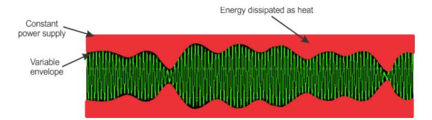
The consequence of the PA inefficiency is very practical. The smart phones will be hotter and their batteries will run out quickly; at the same time, mobile and broadcast network operators need to pay a lot for the wasted energy.
