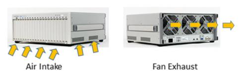
The M9018A/M9018B/M9019A has multiple air intakes. They are located at the lower sides, lower front, and bottom of the chassis.
