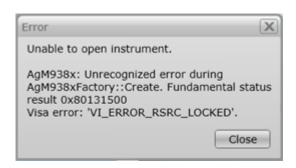
This configuration will retain control of the M9300A if you try to open a new configuration. If you connect a new configuration, that includes the same M9300A, you will see the following error:
