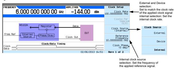
When you select a clock source, you must let the N5102A module know the frequency of the clock signal using the **Clock Rate** softkey. In the internal clock source mode, use this softkey to set the internal clock rate. For device and external clock sources, this softkey must reflect the frequency of the applied clock signal.
