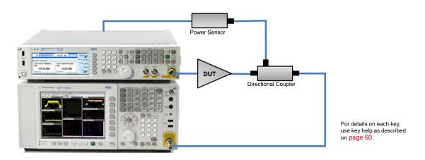
2. Set the signal generator frequency and amplitude to the desired settings for your device.
