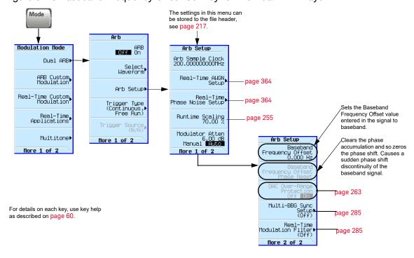
Figure 9-13 Baseband Frequency Offset Softkey for the Dual ARB Player
