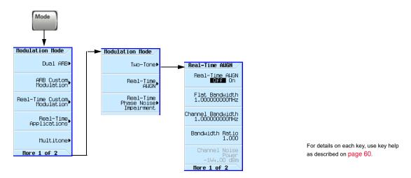
Use the following steps to apply 10 MHz bandwidth noise to a 500 MHz, -10 dBm carrier.
