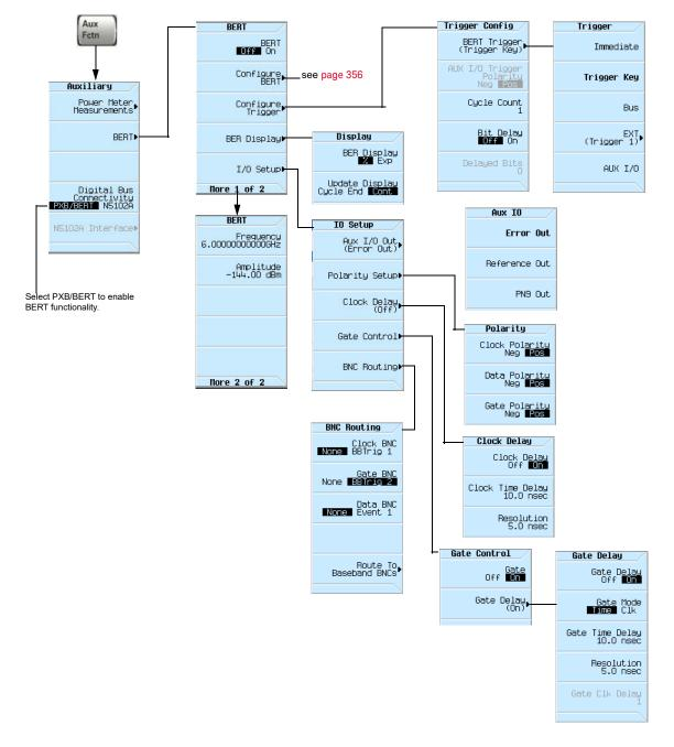
Figure 12-15 BERT I/O Setup Softkeys
