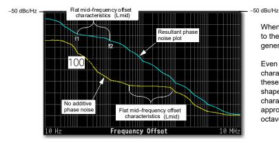
When turned on, this phase noise is added to the base phase noise of the signal generator.
