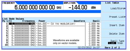
Presetting the list clears any previously selected waveforms.
