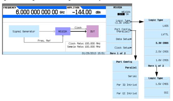
1. Refer to Figure 10-11. Press the Logic Type softkey.
