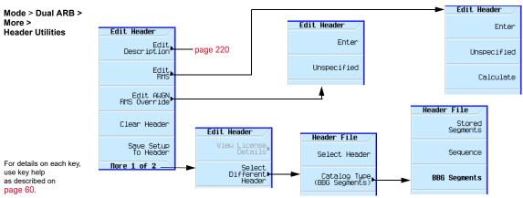
When you create a waveform sequence (as described on page 212), the signal generator automatically creates a waveform sequence header that takes priority over the individual waveform segment headers. During a waveform sequence playback, the segment headers are ignored, except to verify that all required options are installed. Storing a waveform sequence also stores its file header.
