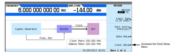
From this softkey menu, set all of the clock parameters that synchronize the data between the N5102A module and the device. From this menu, the clock signal phase can be changed so the clock occurs during the valid portion of the data. Figure 10-20 shows the clock setup menu.
