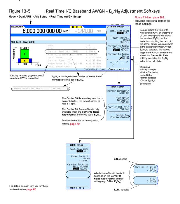
Figure 13-6 Carrier to Noise Ratio Components
