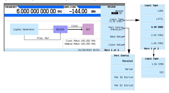
1. Refer to Figure 10-18. Press the **Logic Type** softkey.
