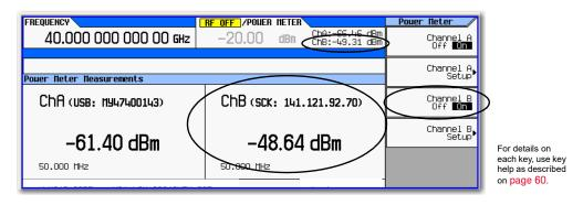
20. The power sensors are now ready to be connected in a measurement setup.
