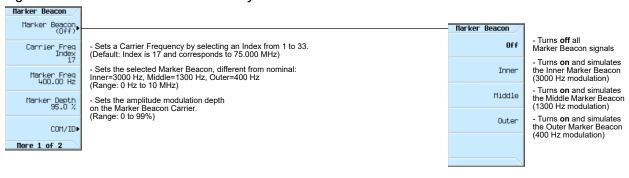
When testing an ILS [Instrument Landing System], the following ILS Marker Beacon parameters can be set:
