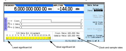
The N5102A module clock rate is set using the **Clock Rate** softkey and has a range of 1 kHz to 400 MHz. The sample rate is automatically calculated and has a range of 1 kHz to 200 MHz. These ranges can be smaller depending on logic type, data parameters, and clock configuration.
