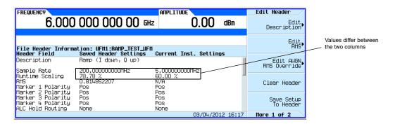
**e.** Save the current settings to the file header: Press the **Save Setup To Header** softkey.
