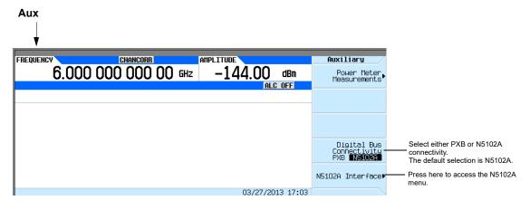
Press N5102A Interface to access the UI (first-level softkey menu shown in Figure 10-10) that is used to configure the digital signal interface module. Notice the graphic in the signal generator display, showing a setup where the N5102A module is generating its own internal clock signal. This graphic changes to reflect the current clock source selection.
