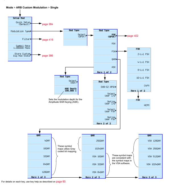
Figure 16-4 Custom Modulation Formats and Applications
