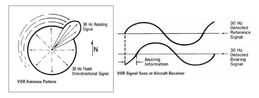
When using an X-Series signal generator with Option N5180302B Avionics License to simulate VOR signals, the 30 Hz reference signal (REF Freq) is placed on a sub-carrier of 9960 Hz (SubCarrier Freq) using frequency modulation with a peak deviation set to 480 Hz (REF Deviation). This frequency modulated sub-carrier is then amplitude modulated onto one of the VOR carriers (108.00 to 117.95 MHz). This makes the reference signal essentially an FM/AM multiplex signal.
