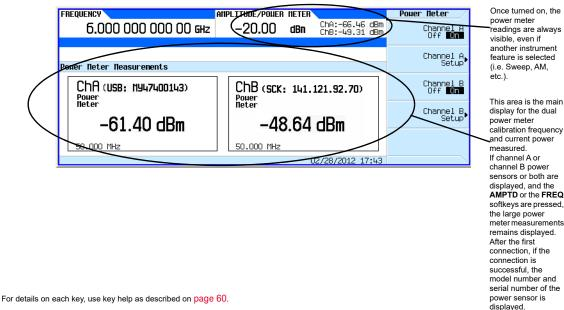
Figure 4-2 Dual Power Meter Display Menu
