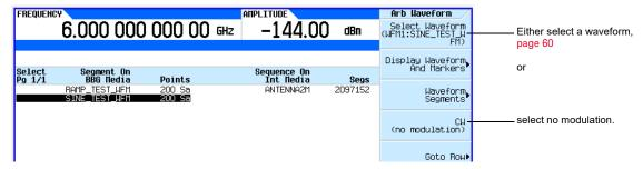
**b.** Highlight the desired waveform (in this example, SINE\_TEST) and press either the **Select** hardkey or the **Select Waveform** softkey.
