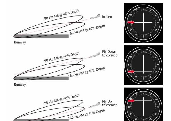
Figure 5-15 ILS Glide Slope @ 334.70 MHz w/ Aircraft In-Line, Fly Down, Fly Up
