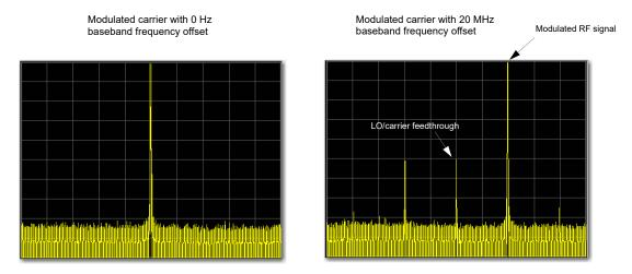
Spectrum analyzer set to a span of 100 MHz
