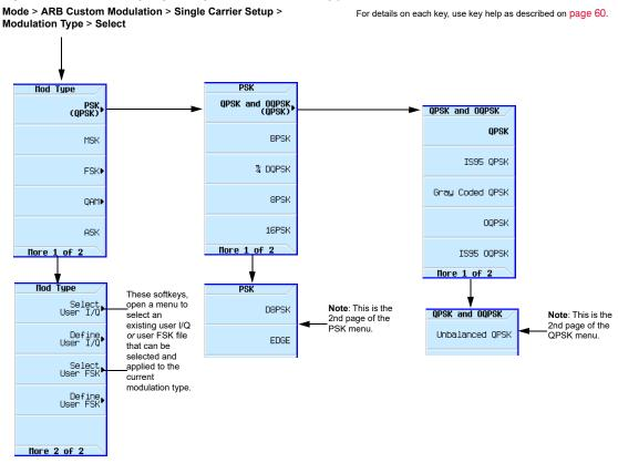
Figure 16-19 Modifying a Digital Modulation Type
