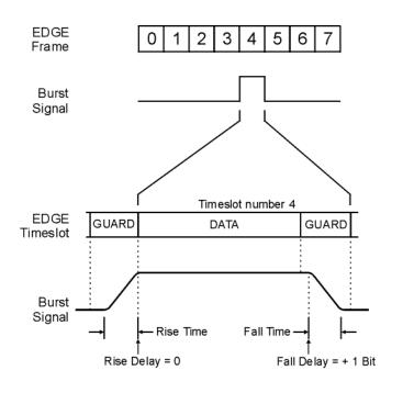
The signal generator firmware computes optimum burst shape based on the settings you've chosen for modulation. You can further optimize burst shape by lining up the data portion with the modulation. For example, if you're designing a new modulation scheme, do the following:
