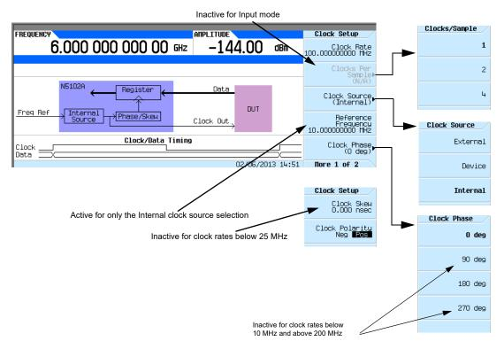
The top graphic on the display shows the current clock source that provides the output clock signal at the Clock Out and Device Interface connectors. The graphic changes to reflect the clock source selection discussed later in this procedure. The bottom graphic shows the clock edges relative to the data. The displayed clock signal will change to reflect the following:
