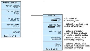
When testing a VOR [VHF Omnidirectional Ranging] or ILS [Instrument Landing System], the following COM/ID parameters can be set:
