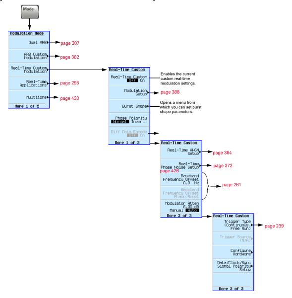
Figure 16-6 Real-Time Custom Modulation Softkeys
