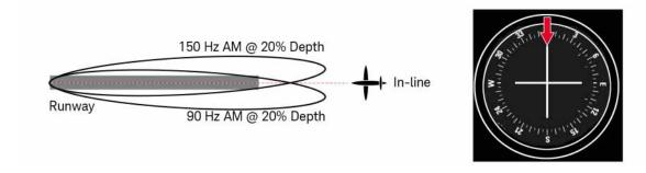
Figure 5-12 ILS Glide Slope: 334.70 MHz w/ 90 Hz AM (Up), 150 Hz AM (Down) @ 40%
