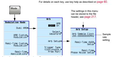
rate. The location of the sample rate setting is shown in the figure at right.
