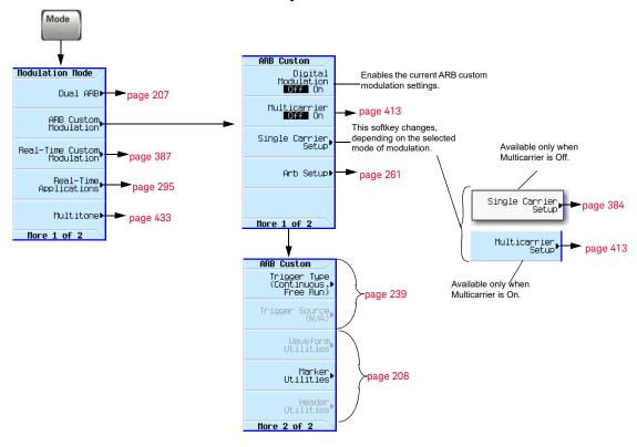
Figure 16-1 ARB Custom Modulation Softkeys
