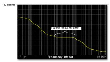
The Keysight X-Series vector signal generator demonstrates a definitive shape to its phase noise plot. The mid–frequency offsets are characterized by a leveling (flattening) of the phase noise amplitude from approximately a 3 kHz offset to approximately a 70 kHz offset.
