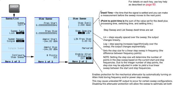
When the attenuator protection is disabled, the step dwell time will be set to a minimum of 50 ms as a precaution.
