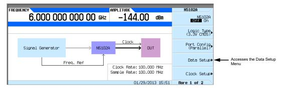
This softkey menu accesses the various parameters that govern the data received by the signal generator. The status area of the display shows the number of data lines used for both I and Q along with the clock position relative to the data. Figure 10-22 shows the data setup menu structure.
