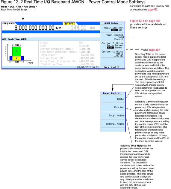
Figure 13-2 Real Time I/Q Baseband AWGN - Power Control Mode Softkeys
