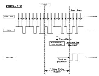
In this example, the triggering sequence is where the trigger delay is active with a cycle count.
