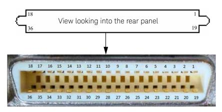
The AUX I/O connector is a shielded .050 series The AUX I/O mating connector manufacturer's part number is 3M® 10136-3000 (wire mount plug).
