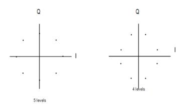
Figure 16-28 16QAM I/Q Map with Even and Uneven Levels
