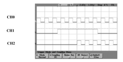
CH0: BER CLK IN (rear panel BNC connector labeled BB TRIG 1) CH1: BER GATE IN (rear panel BNC connector labeled BB TRIG 2)
