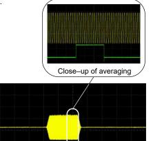
The ALC samples the waveform when the marker signal goes high, and uses the average of the sampled waveform to set the ALC circuitry.
