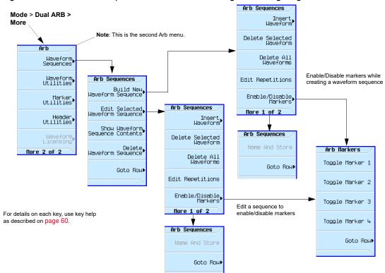
Figure 9-6 Waveform Sequence Menus for Enabling/Disabling Segment Markers
