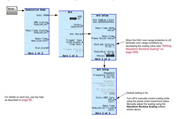
Figure 14-3 Dual ARB DAC Over-Range Protection Softkey Location
