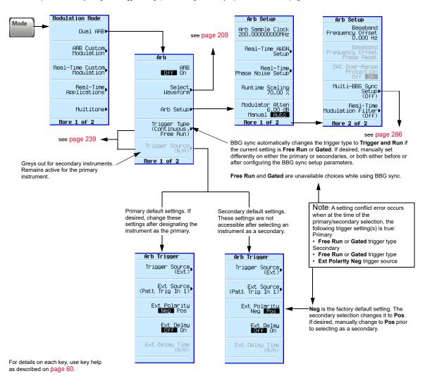
Figure 9-28 Multiple BBG Synchronization Front Panel Displays
