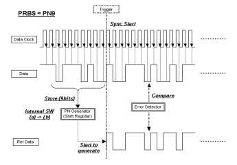
In this example, synchronization occurs after receiving a trigger.
