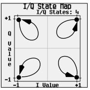
When applied to the user-defined default 4QAM I/Q map, starting from the 1st symbol (data 00), the differential encoding transitions for the data stream (in 2-bit symbols) 0011100001 appear in the following illustration.
