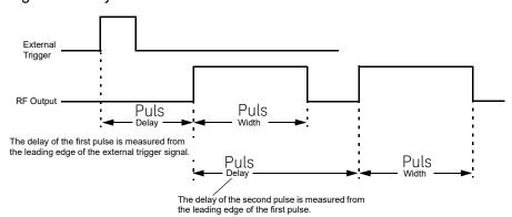
Figure 7-3 Trigger Doublet
