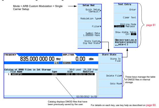
Figure 16-20 Storing a Custom Digital Modulation State
