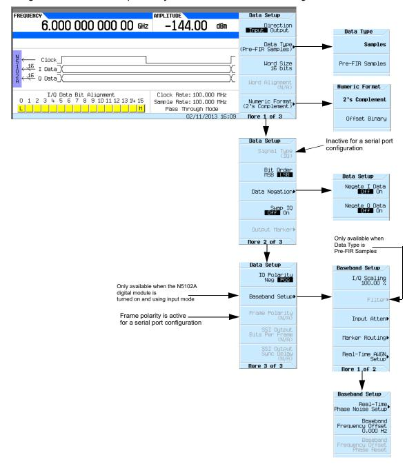
Figure 10-22 Data Setup Softkey Menu with Parallel Port Configuration
