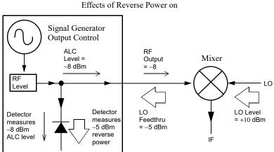
Depending on frequency, it is possible for most of this LO feedthrough energy to enter the detector. Because the detector responds to its total input power regardless of frequency, this excess energy causes the ALC to reduce the RF output. In this example, the reverse power across the detector is actually greater than the ALC level, which can result in loss of signal at the RF output.
