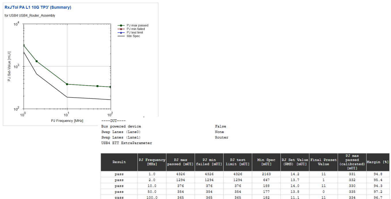
Figure 11. Jitter Tolerance Characterization test results
