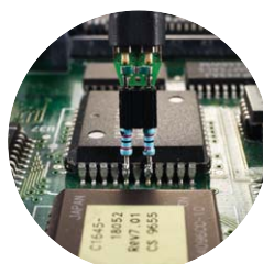
Figure 22. InfiniiMax 7 GHz differential socketed probe head.
