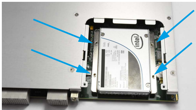
Figure 8 Use M2.5x5 mm screws to mount drive to motherboard
