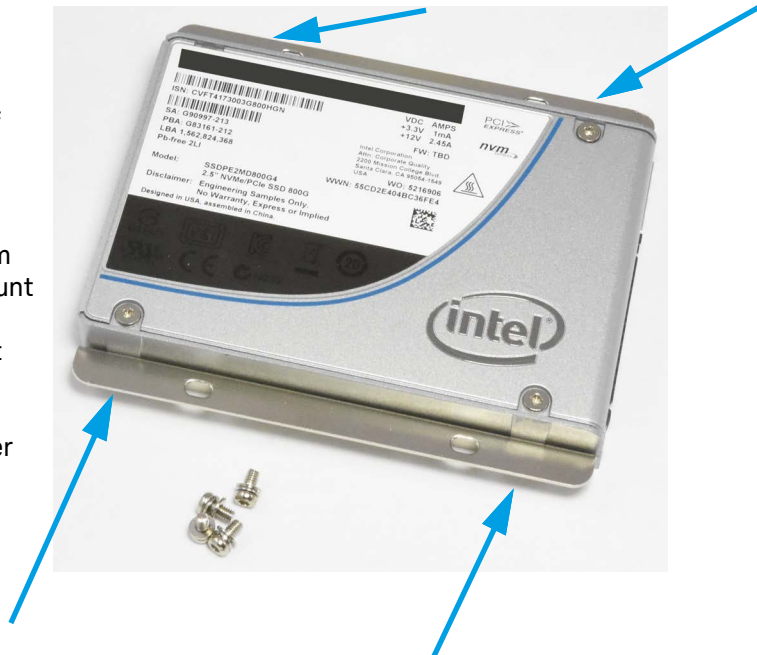
Figure 7 Install Mounting Rails to NVMe Drive
