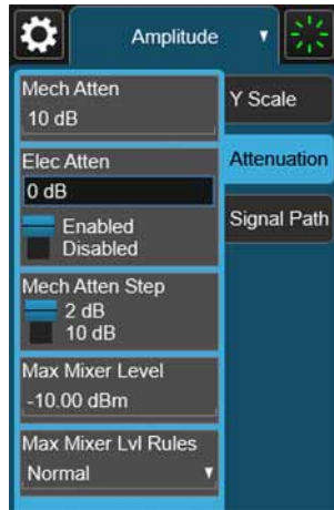
Figure 10-6 A13A1 Electronic Atten Control
