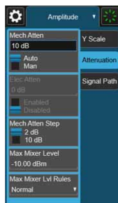
Figure 9-7 A9 and A10 Attenuator Control
