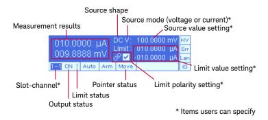
The Meter view has five layout types. To show the single-channel layout, press the **Meter** key until the single-channel layout appears.
