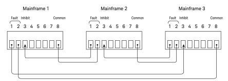
The protection state and the fault output on the digital I/O terminal remain active even if the module emergency condition is released. Users need to disable the protection state explicitly by the :OUTPut:PROTection:CLEar command.
