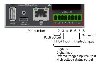
Table 3-3 Pin Configuration for Digital I/O Connector on the Rear Panel
