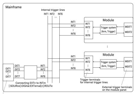
External trigger inputs/outputs (Digital I/O terminals on the mainframe rear panel)
