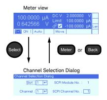
The PZ2100A has two expressions for indicating a channel. One is the slot-channel for the front panel operation, and the other is the channel number for the SCPI programming. You can specify the slot and channel numbers or the channel number for the SCPI programming in the Channel Selection Dialog.
