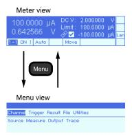
Meter view displays output settings, measurement results, and the status of modules and the mainframe. For more information, see "Meter View and Operation" on page 99.
