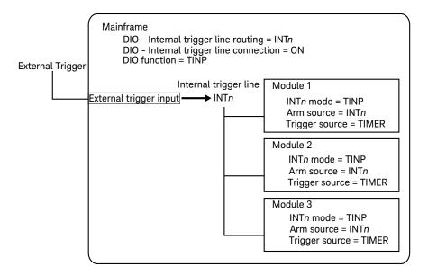
You need only a cable connecting to the external trigger source and the trigger input terminal.
