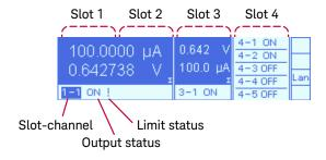
The PZ2110A module occupies two slots, and the module information is displayed on half of the LCD in the same way as the 2-channel layout. A  $\Sigma$  mark on the right-bottom corner means that it is a component of the slot summary, not the 2-channel layout.
