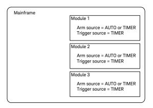
The delay between the modules will be 100 nanoseconds or less.
