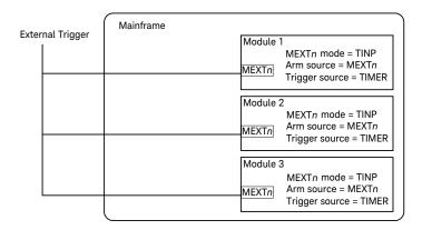
This operation allows you to easily synchronize the modules with other instruments.
