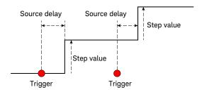
Acquire device action (for voltage or current measurement)
