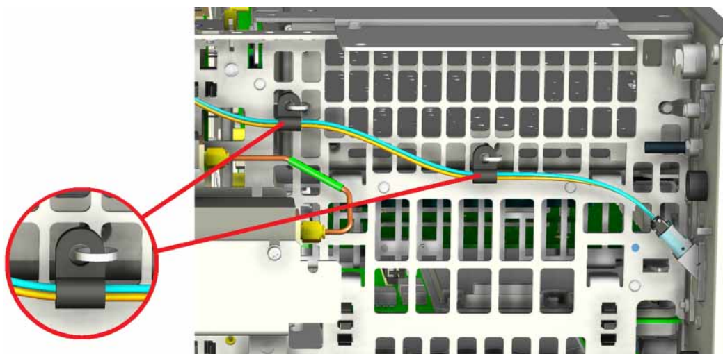
Figure 25 Secure ODI Cable to Chassis
