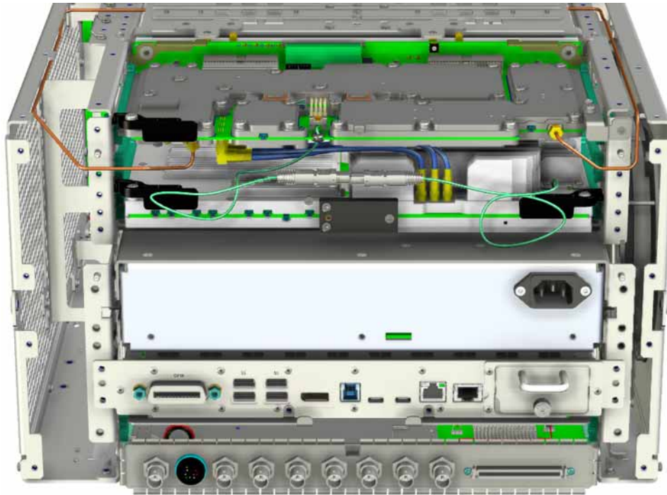
Figure 10 A22 Ultra-Wideband Analog IF Removal - Option R40
