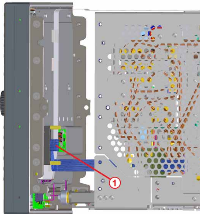
Figure 5 W2 Access and Removal
