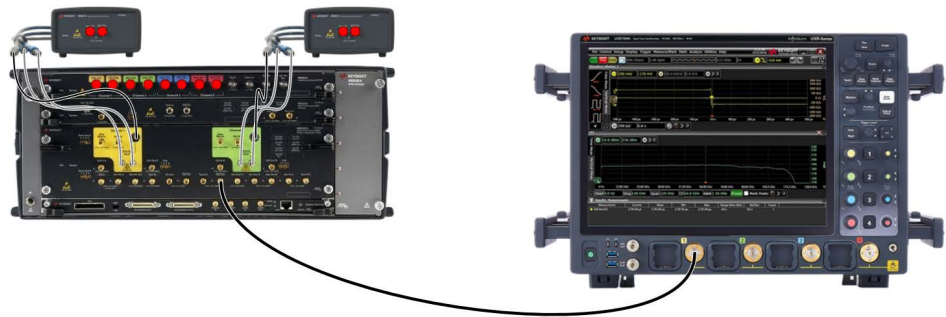
Figure 4-9 Example connection diagram for Reference Clock Calibration (M8040A)
