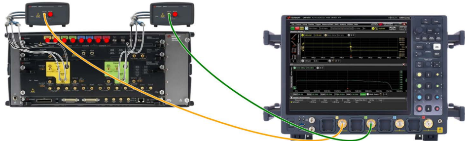
Figure 4-24 Example connection diagram for Inter Pair Skew Calibration (M8040A)
