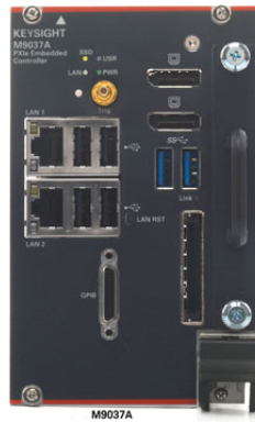
Figure 6 Front panel view of M9037A Embedded Controller
