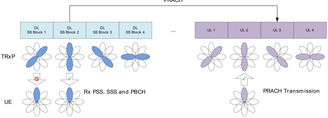
Same Tx beam direction as in the DL Tx beam
