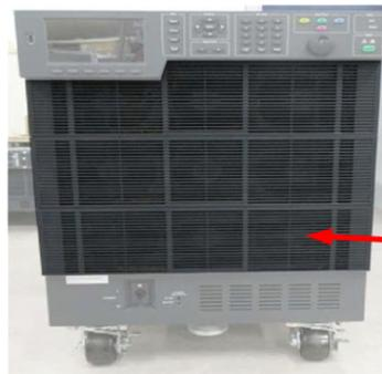
2. Start by pinching the center projection part of the louver and pulling the louver forward.
