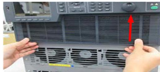
3. Press the lock pins on both sides of louver into the holes on the power unit.
