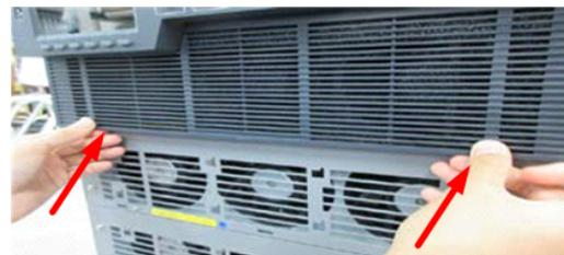
4. Press the lock pin in the center of the louver into the center hole on the unit.
