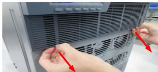
4. Slide the louver downward, and remove the louver.
