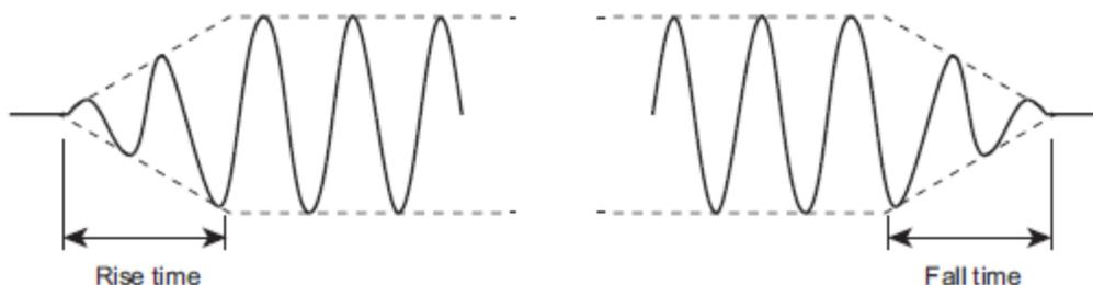
Soft start and stop cannot be set when the product is being controlled with an external analog signal and the signal source is set to external signal (EXT) only or when the product is being controlled with an external analog signal and the voltage is being varied using an external DC signal. Soft start and stop are disabled when the current limit is exceeded.
