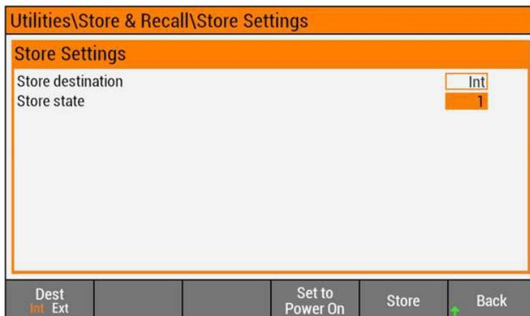
Toggle the **Destination** softkey to select either an Internal or External storage location. When the destination is Internal, you have the option of selecting from 0 to 9 internal storage locations. Specify the location in the Store state box.
