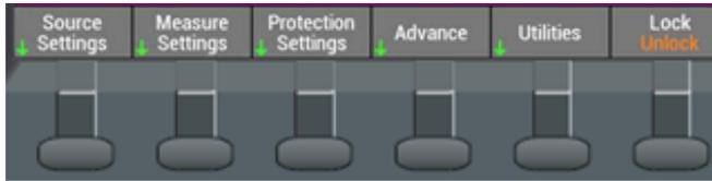
The green down arrows are used to indicate that there is a lower level within that menu. If there is no more down arrow, it indicates that you are at the lowest possible level. The Green up arrow is used to move back to the upper level.
