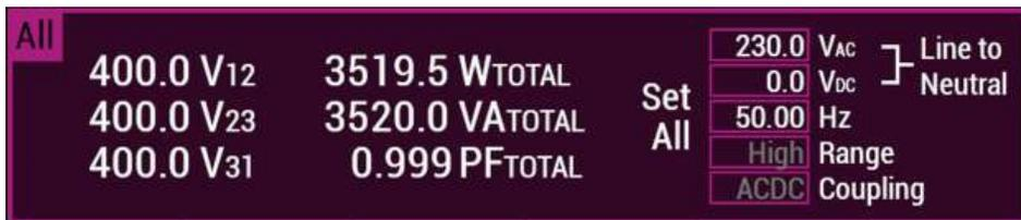
The **All** area of the display shows the measurements that apply to all phases. On the left side, the line-to-line voltage between the indicated phases is shown (phase 1 to 2, 2 to 3, and 1 to 3). The right side of the display shows the line-to-neutral voltage, provided it is the same for all phases. It also displays the total power in Watts, the apparent power in VA, and the power factor.
