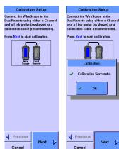
**Note<sup>3</sup>:** You will be prompted a message if the DualRemote Pro is detected to have different version of firmware compare with the WireScope<sup>TM</sup> Pro Main unit. Just confirm if you want to proceed with calibration to upgrade the DualRemote's firmware.
