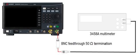
RG58 coaxial cable with BNC (m) to dual banana adapter
