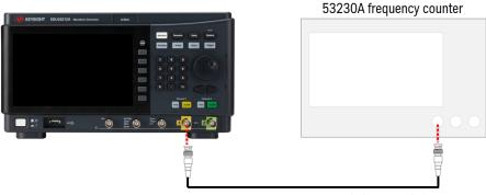
RG58 coaxial cable with BNC (m) to BNC (m)
