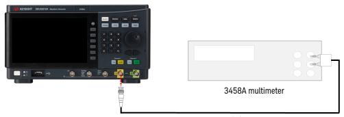
RG58 coaxial cable with BNC (m) to dual banana adapter
