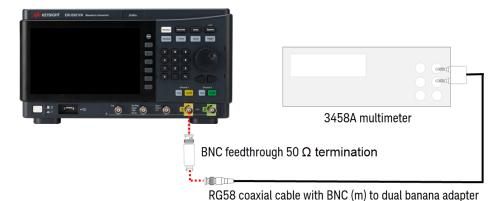
2. Set the instrument to each output in the table below and configure the multimeter to AC mode. Measure the output voltage with the multimeter. This will become the reference measurement. Set the output impedance to 50 Ω. Be sure the output is enabled.
