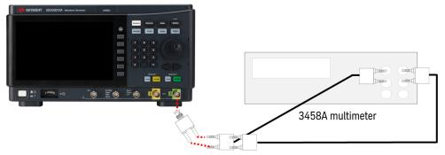
RG58 coaxial cable with BNC (m) to dual banana adapter
