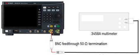
RG58 coaxial cable with BNC (m) to dual banana adapter
