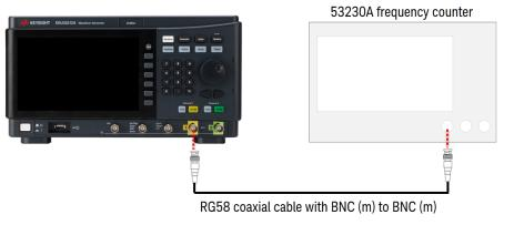
2. Set the instrument to the output described in the table below and measure the output frequency. Be sure the instrument output is enabled.
