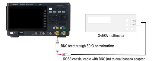
2. Configure 3458A multimeter to ACV mode and measure the output for each setup in the following table.
