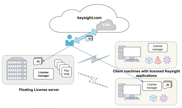
The floating license server, on the left, provides licenses for the two clients at the right; the second client also has node-locked licenses for use on that machine only. When the applications (shapes) are run, they request licenses, which are provided from any available location by the licensing software. When users install new Keysight software, they also get a license manager utility that helps them install and manage their licenses.
