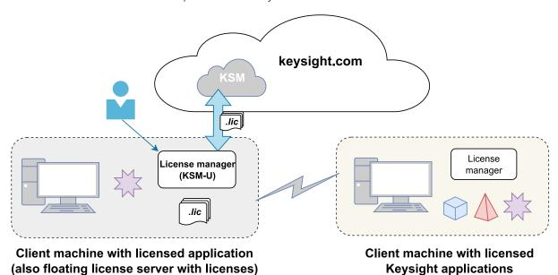
With Easy Activation the user enters an activation code from their Keysight entitlement certificate into the activation wizard in KSM-U. That triggers a license request between KSM-U and the KSM website. Assignment of a host ID to the license is handled automatically, as is installation of the activated license on the host machine.
