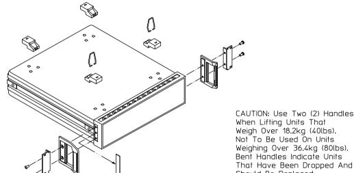
Weighing Over 36.4kg (80lbs). Bent Handles Indicate Units That Have Been Dropped And Should Be Replaced.
