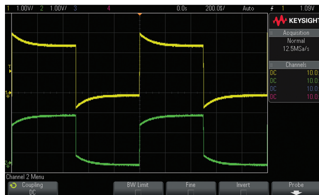
Figure 3: Improperly compensated probes.
