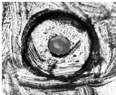
Figure 1-6. Damage from improper cleaning.
