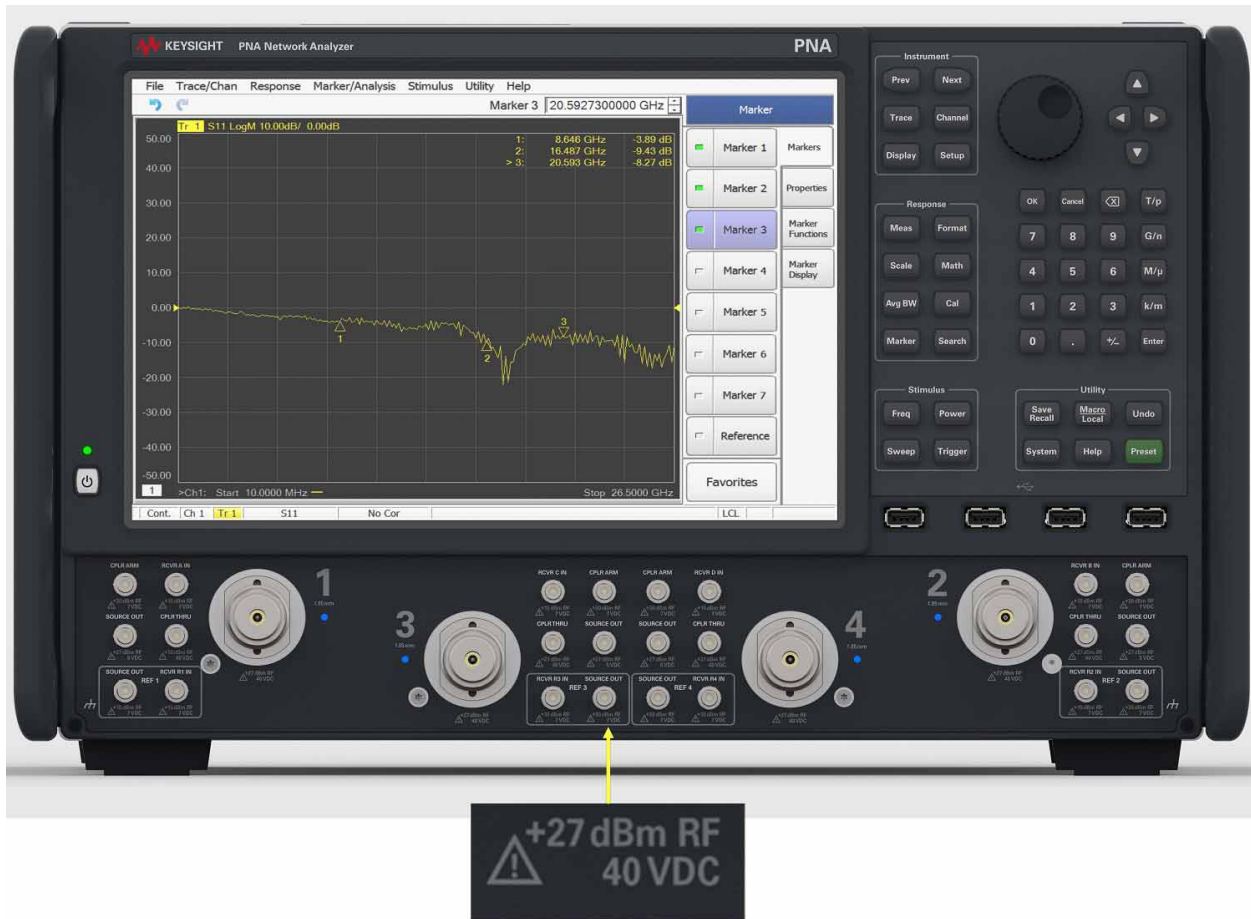
Figure 1 Example Label Showing Damage Level for Each Port and Connector
