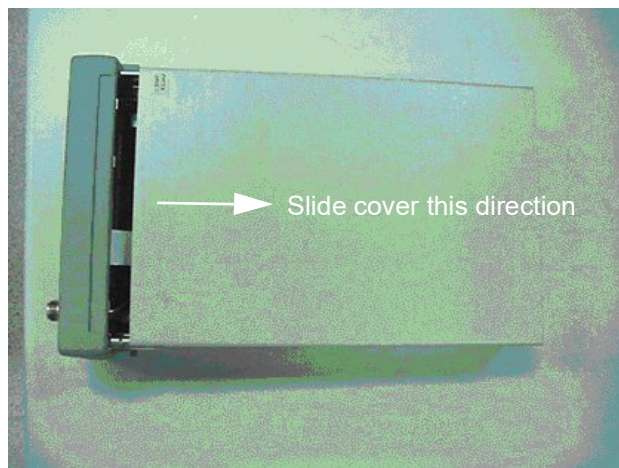
Figure A-3 Remove the power meter cover
