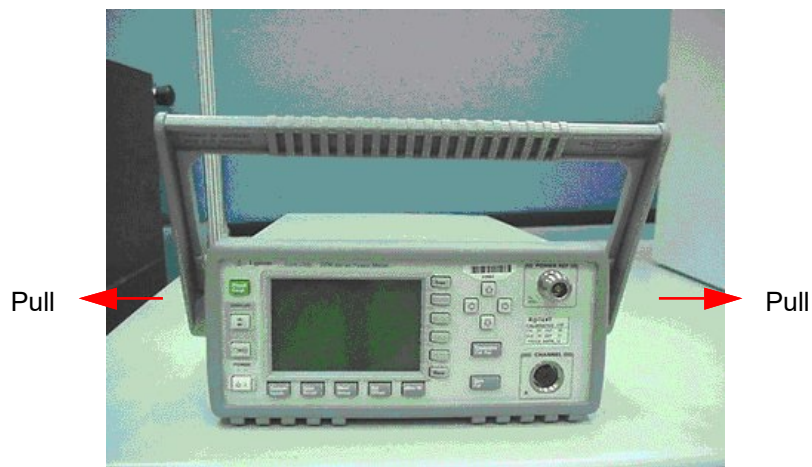
Figure A-2 Remove the power meter handle
