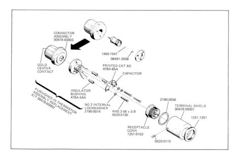
Figure 4-4 Model 478A Thermistor Mount Assembly
