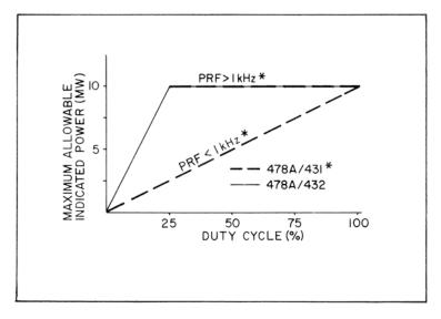
**Figure 2-2** Maximum Power Meter Reading vs Duty Cycle for Pulses Longer than 250 μs
