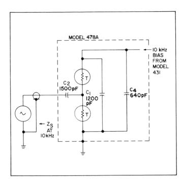
Figure 2-4 Source Impedance Shunting One RF Thermistor Mount
