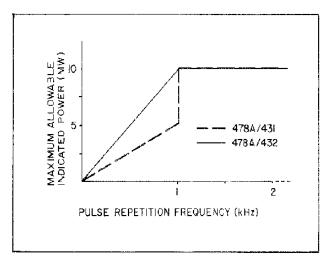
Figure 2-1 Maximum Power Meter Reading vs PRF for Pulses Shorter than 250  $\mu s$
