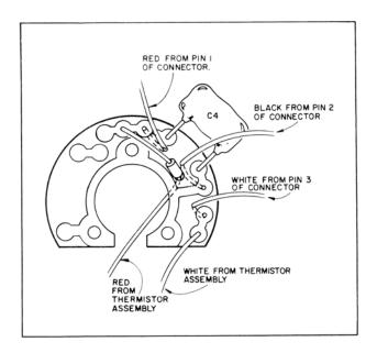
Figure 4-5 Keysight Model 478A Printed Circuit Assy Wiring
