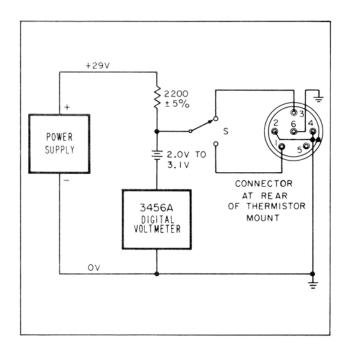
Figure 4-2 Check on Model 478A Thermistor Resistance Match
