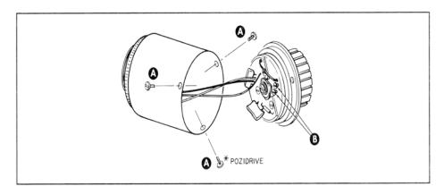
Figure A-7 Thermistor Compensation (P/O Change B)
