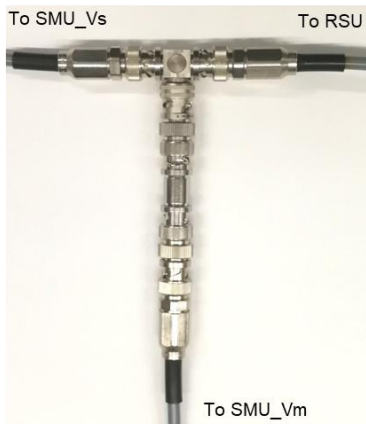
Figure 2-6. Triax TEE configuration using adapters.
