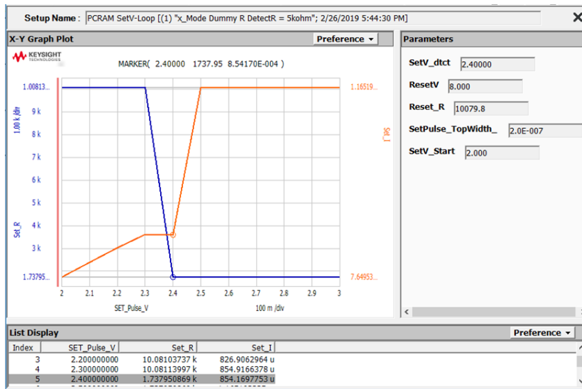
Figure 2-31. PCRAM SetV-Loop measurement example.
