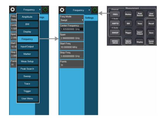
Notice that the Frequency panel has a Settings tab on the right side. Other panels may have multiple tabs. The tabs access controls for the particular parameter noted on the tab.
