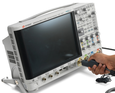
Figure 4 Connecting the Probe to the Oscilloscope
