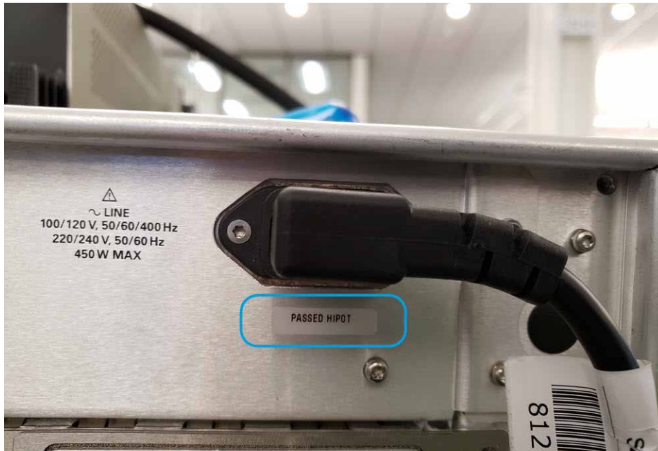
Hi-Pot Sticker on the Power Supply Cover
