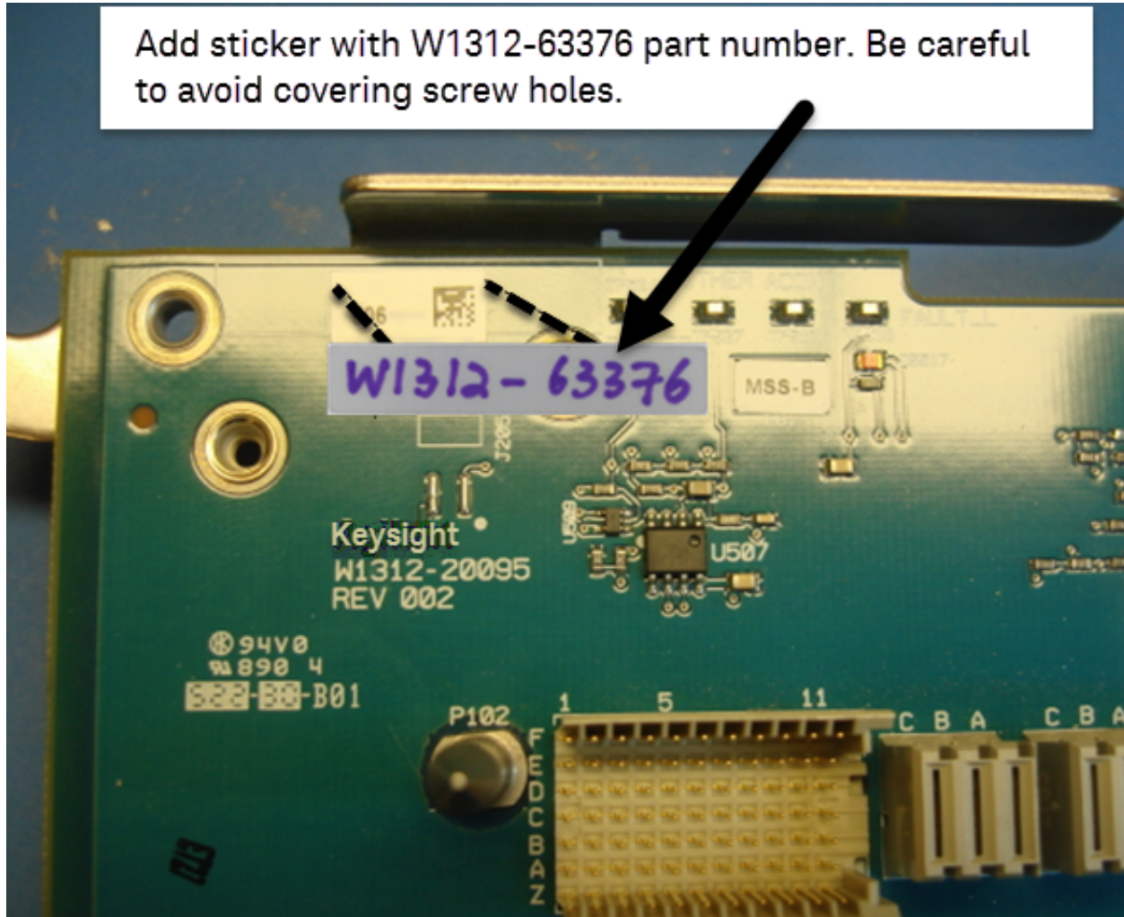
Figure 0-6 Adding sticker to new board number W1312-63376—Top Side View
