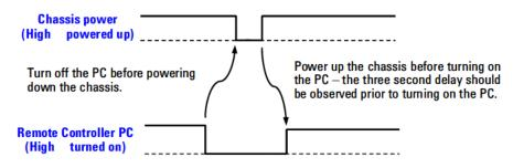
Figure 12 Power Sequence for a System Restart
