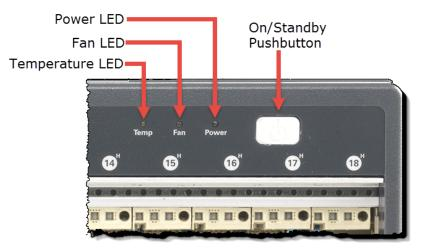
Figure 7 Chassis Front Panel LEDs
