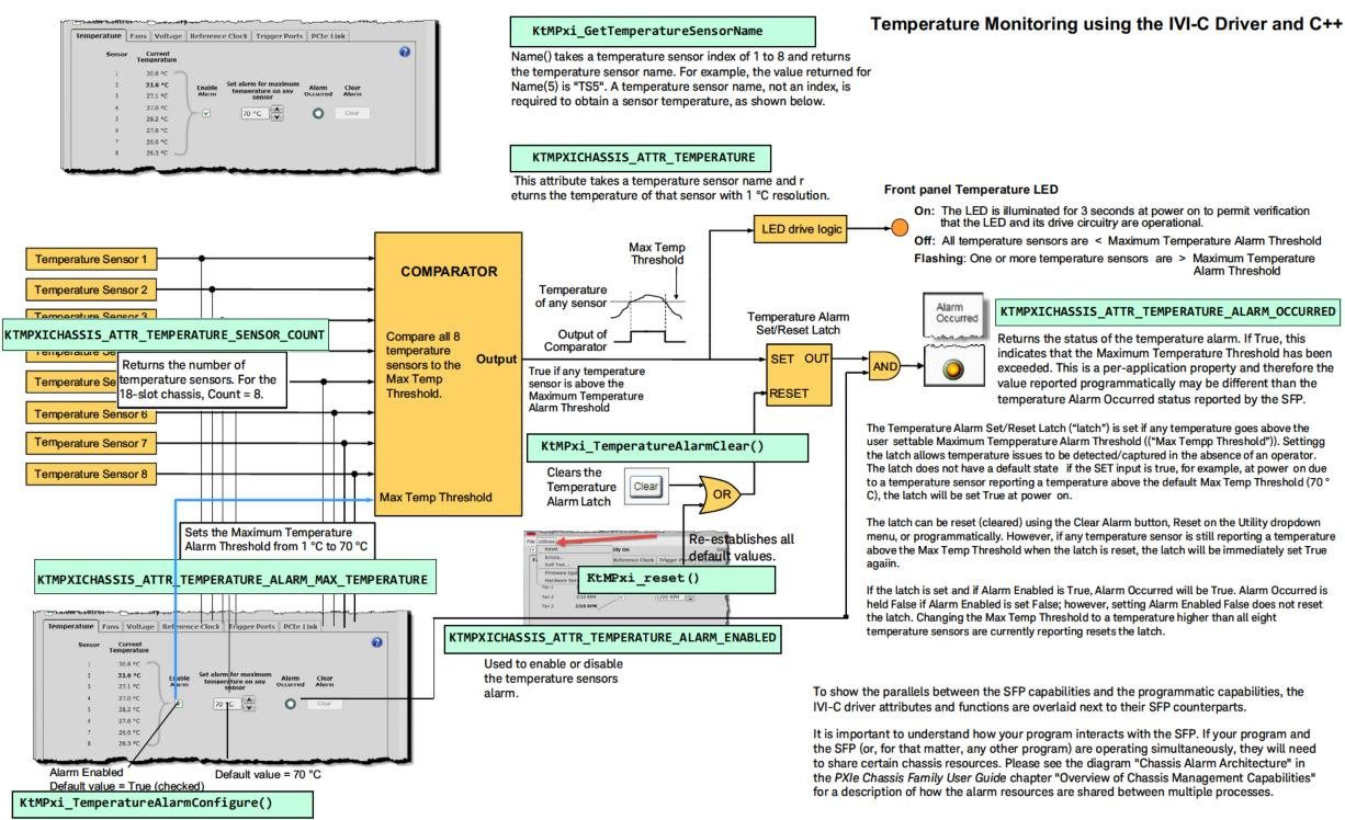
Configures the temperature alarm behavior by allowing setting of both the Maximum Temperature Alarm Threshold (MaxTemperature) and the Enabled property.
