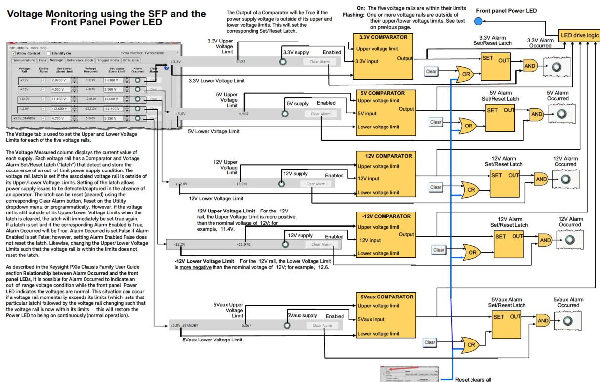
Figure 18 Using the Soft Front Panels to Monitor Chassis Power Supply Rails
