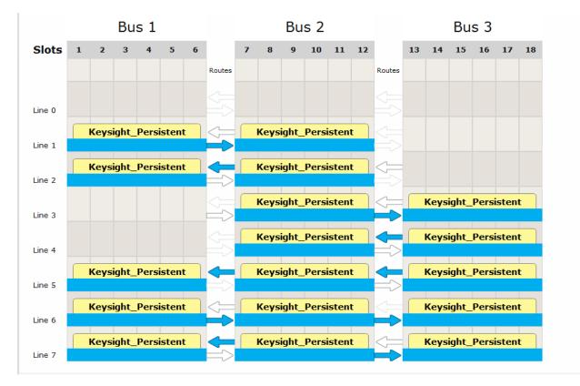
Figure 38 Example Showing the Eight Different Triggering Bus Routes
