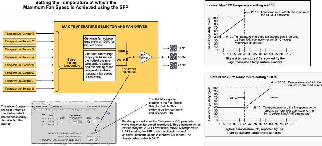
The PXIe chassis controls the speed of its three fans by varying the duty cycle of the drive voltage to the fans. When the rear panel FAN switch (referred to as the "Fan Speed Selector Switch") is set to HIGH, the fan voltage duty cycle is set to 100%, which generates the highest fan speeds and the best chassis cooling however, this also generates the most fan noise.
