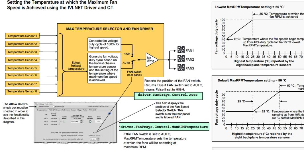
The PXIe chassis controls the speed of its fans by varying the duty cycle of they drive voltage to the fagns. When the rear panel FAN switch (referred to as the "Fan Speed Selector Switch") is set to HIGH, the fan voltage duty cycle is set to 100%, which generates the highest fan speeds and the best chassis cooling however, this also generates the most fan noise.
