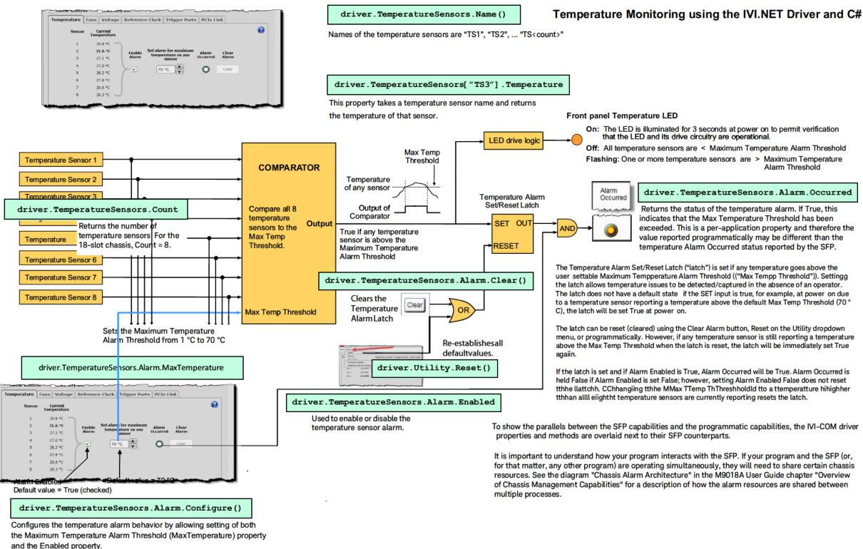
Figure 27 Temperature Monitoring using the IVI.NET Driver and C#
