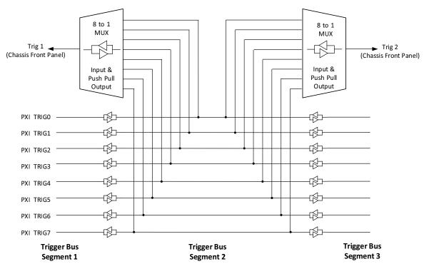
Figure 46 Wiring diagram illustration of an example front panel Trigger Port configuration.
