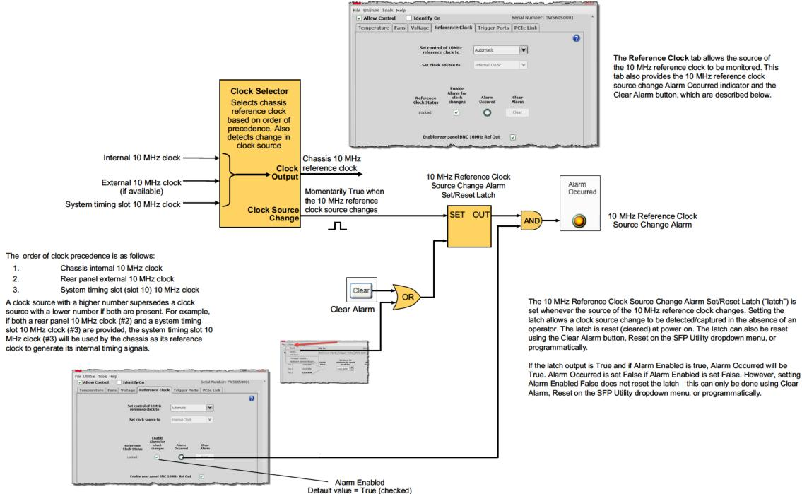
10 MHz Reference Clock Source Monitoring Using the SFP
