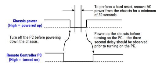
Figure 13 Power Sequence for a Chassis Hard Reset
