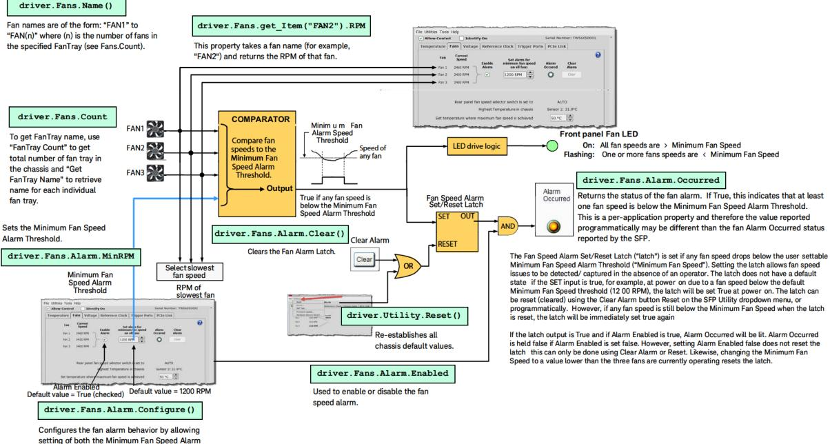
Figure 30 Chassis Fan Speed Monitoring using the IVI.NET Driver and C#
