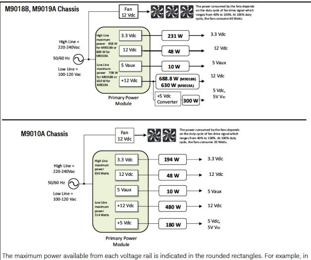
The maximum power available from each voltage rail is indicated in the rounded rectangles. For example, in the M9018B and M9019A chassis, the maximum power available from the 3.3 Vdc rail is 231 W and the maximum power available from the 5 Vdc rail is 300 W. The sum of all of the wattages cannot exceed the maximum power available from the Primary Power Module (PPM).
