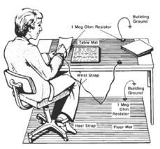
Both types, when used together, provide a significant level of ESD protection. Of the two, only the table-mat and wrist-strap combination provides adequate ESD protection when used alone. To ensure user safety, the static-safe accessories must provide at least 1 M $\Omega$  of isolation from ground.
