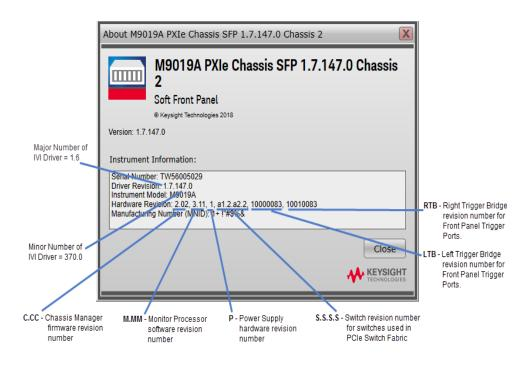
Figure 74 Chassis Firmware Shown in the Soft Front Panel (M9019A shown)
