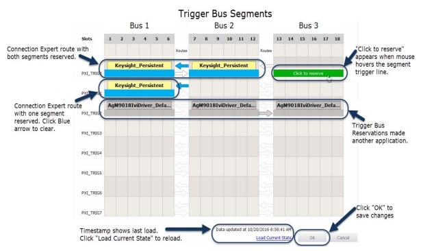
**Figure 37** Keysight IO Libraries Connection Expert Chassis Triggers View (M9018B and M9019A)
