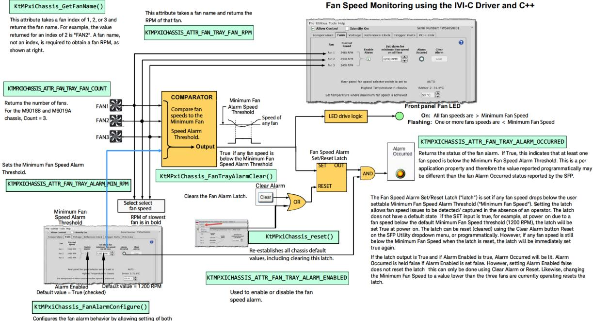
Figure 29 Chassis Fan Speed Monitoring using the IVI-C Driver and C++
