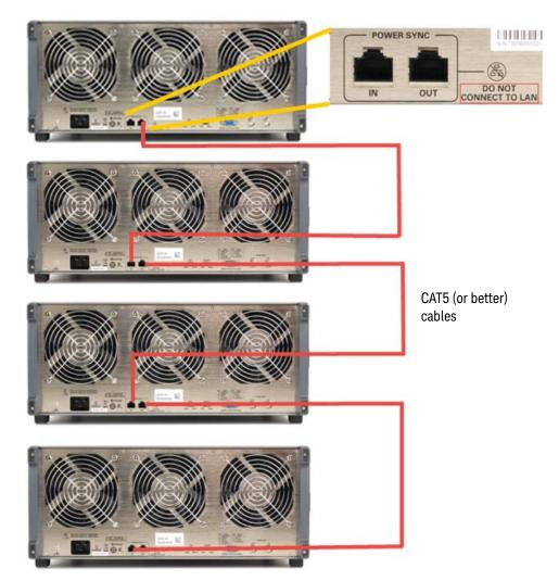
Figure 55 Connection Sequence for Multiple Chassis Power Synchronization
