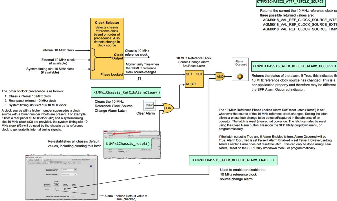
Figure 35 10 MHz Reference Clock Source Monitoring using IVI-C and C++
