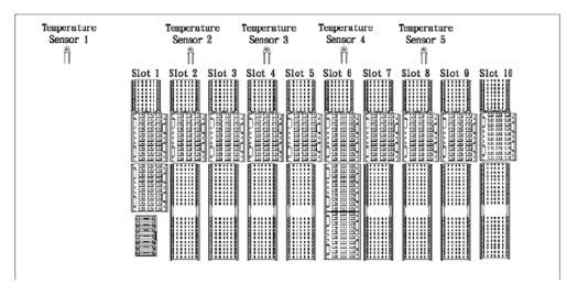
Figure 24 Temperature Sensor Locations in M9010A Chassis.
