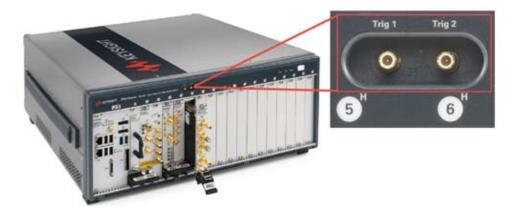
Figure 3 Chassis Front Panel Trigger Ports (M9019A shown)
