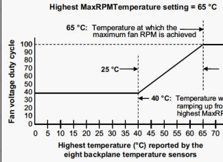
Figure 33 Setting the temperature for Maximum Fan Speed using the IV.NET Driver and C#
