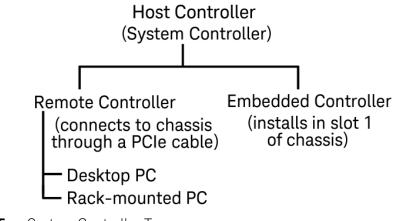
Figure 5 System Controller Types
