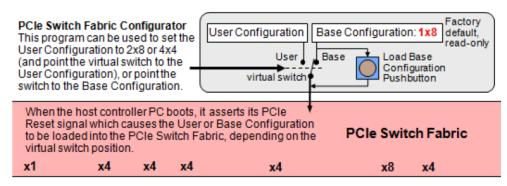
Figure 60 User and Base Configurations
