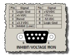
Figure 17 DB-9 Connector Pin-out from Chassis Rear Panel
