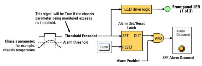
Figure 15 Example Alarm Latch and Front Panel LED
