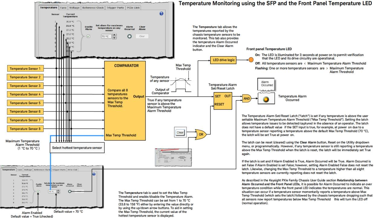
Figure 25 Using the Soft Front Panel to monitor Chassis Temperature
