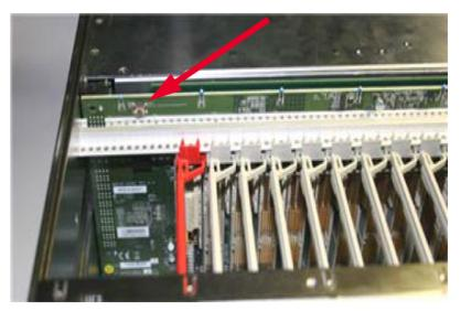
Figure 71 Load Base Configuration Pushbutton (M9018A only)
