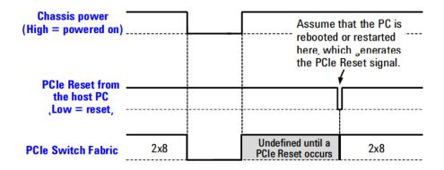
This diagram shows the status of the PCIe Switch Fabric across a chassis power cycle. In this example, the PCIe Switch Fabric is set to 2x8. When the chassis is powered down and powered back up, the PCIe Switch Fabric is, as usual, undefined until a PCIe Reset signal occurs.
