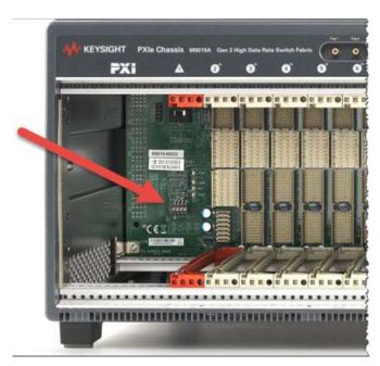
Figure 75 PXIe Chassis Backplane Switches
