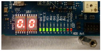
Figure 4 LEDs on CPU module
