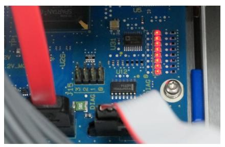
Figure 5 LEDs on DSP module
