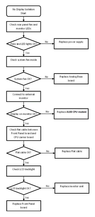
Figure 3 No display trouble isolation procedure
