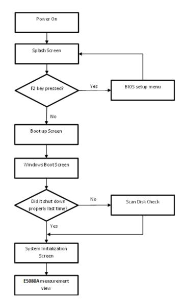
Figure 7 Booting process flowchart
