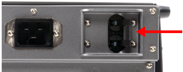
Figure 18 Chassis circuit breaker
