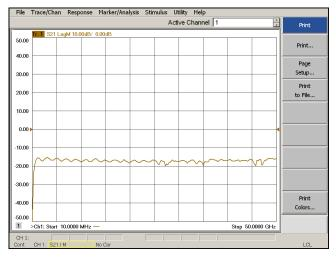
Connect the RF Flex cables to the Source IN and CPLR THRU port indicated in Table 21, the expected results should be similar to Figure 60.
