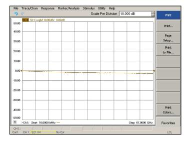
Connect the RF Flex cables to the Source IN and CPLR ARM port indicated in Table 22, the expected results should be similar to Figure 60 on page 84.
