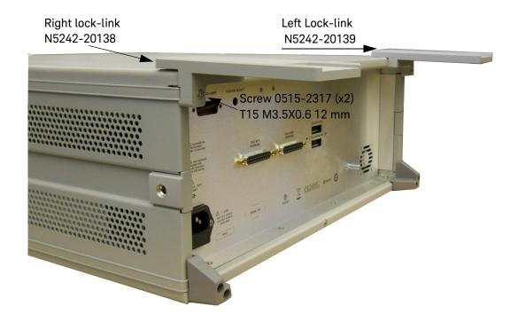
7. Place the analyzer on top of the test set and ensure that the front frame of the analyzer is positioned slightly forward of the locks that are attached to the test set. Slide the analyzer back so the locks engage the front frame of the analyzer.
