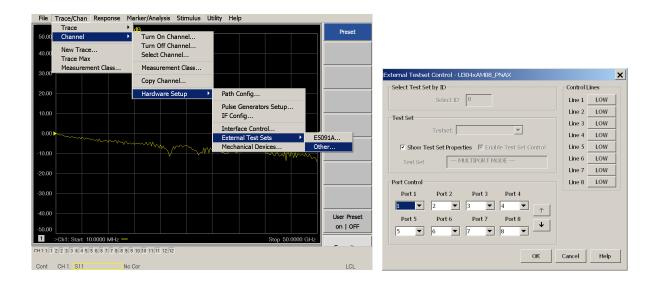
This menu will allow the physical Ports 1 thru 16 to be identified as any port for your convenience. For example, Port 5 can be re-named Port 2.
