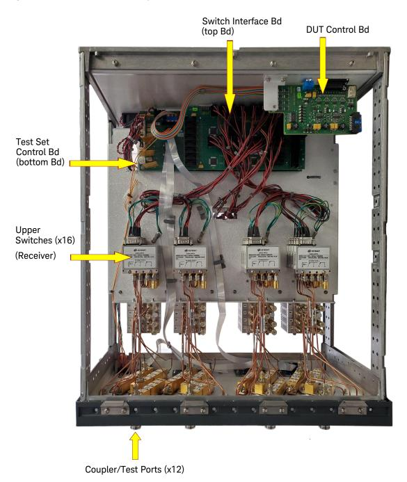
Figure 62 Test Set Bottom View
