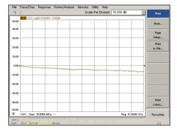
Figure 56 Source IN to Ports 13 to 16 Path Response
