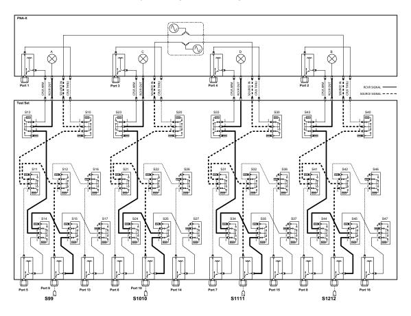
Figure 18 Typical Reflection Response Ports 13 to 16
