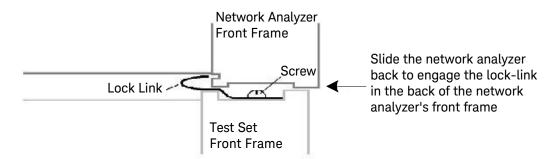
8. Secure the analyzer's lower lock-links to the test set's upper lock-link using the spring-loaded screws. If the analyzer's lock-links are not aligned with the screw holes, loosen the screws securing the feet to the instrument to align and tighten.
