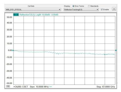
Figure 47 Typical Reflection Tracking (Ports 9 to 12)
