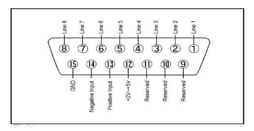
Table 12 DUT Control Line Interface Connector Pin Assignment
