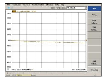
Figure 55 Source IN to Ports 9 to 12 Path Response
