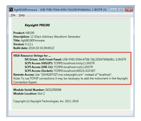
Step 3 - Now change the properties of the two newly created shortcuts. You need to add new parameters to the target string. Copy the Visa Resource String for first firmware and add it to the target field and press "OK".
