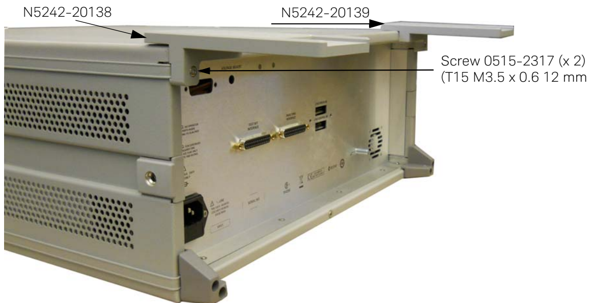
Figure 7 Install Locking Feet on Test Set
