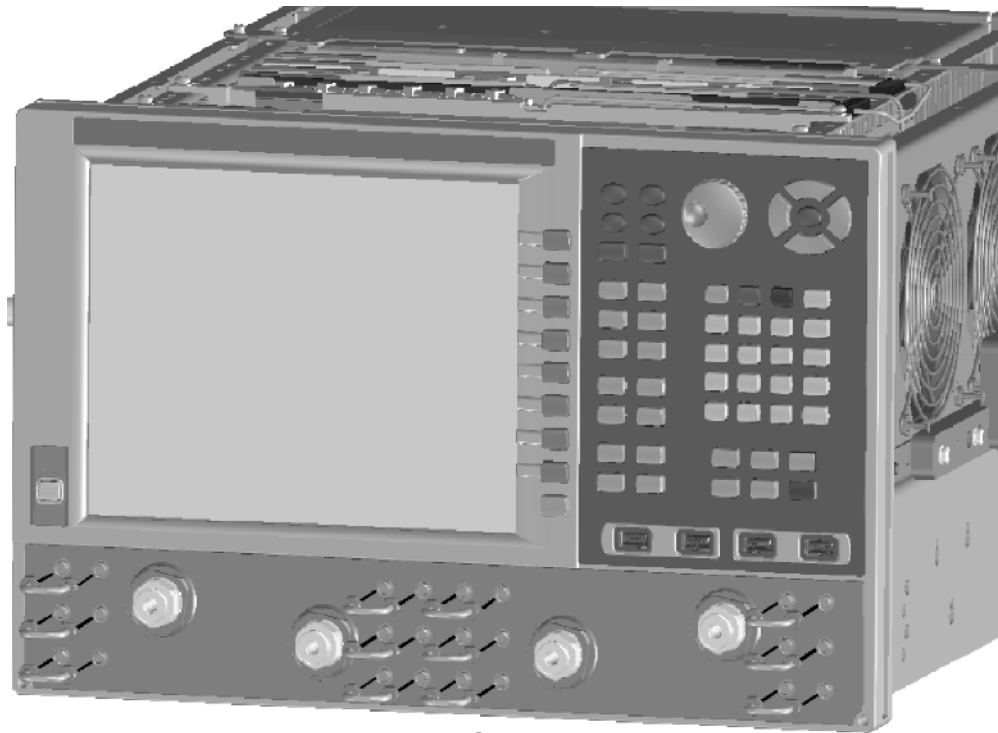
Figure 5 Front Panel Jumper Cables Installation
