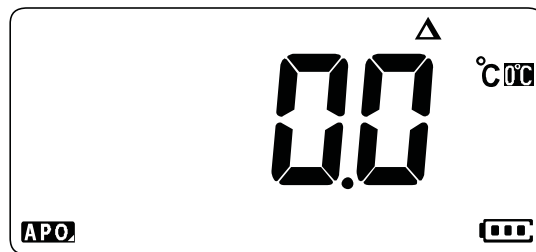
Figure 2-21 Temperature measurement without ambient compensation
