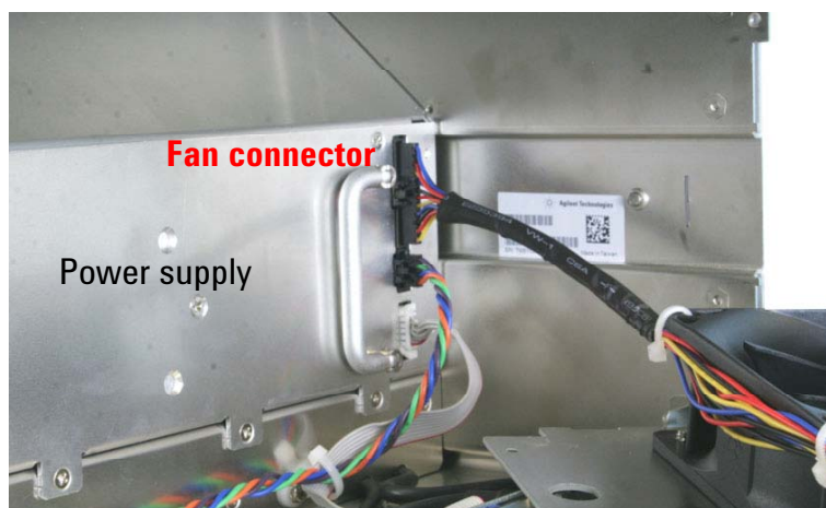
Figure 82 The fan connector is the top-most connector.
