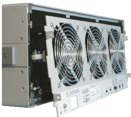
Figure 80 Removal of the rear panel
