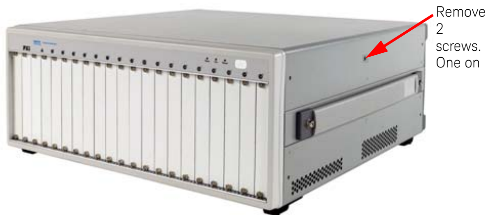
Figure 87 Remove screws on side of chassis
