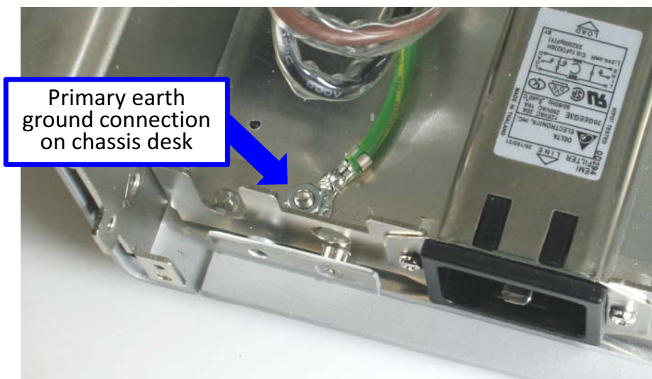
Figure 96 Measure the resistance from the power supply enclosure to the primary earth ground connection on the chassis deck.
