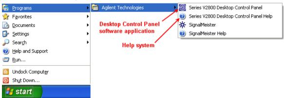
See the "Controlling the Instrument via Desktop Control Panel" topic group in the Series V2800 help system for information about operating the software.
