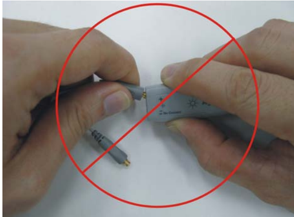
Figure 1-2 An improper way to disconnect a probe head from an amplifier
