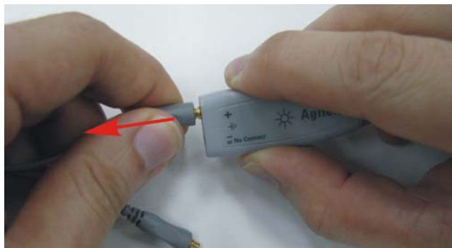
Figure 1-1 Pull the probe head straight out to disconnect it from the amplifier.
